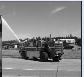
After replacing water pump clutch assembly on one of Whidbey's T-1500 Oshkosh crash trucks, Heavy Equipment Mechanic, Steve Whalen tests the pump, roof turret, and bumper turrets on this critical piece of emergency equipment. ✦
